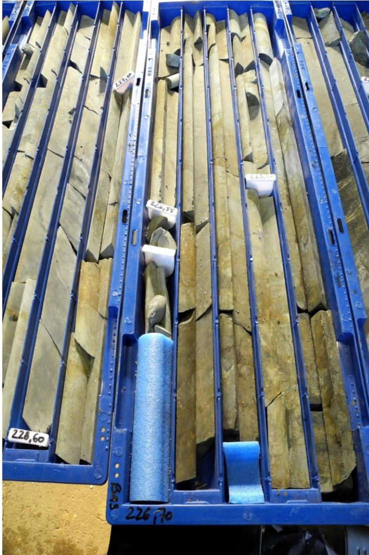
Massive sulfide zone in PAM5
